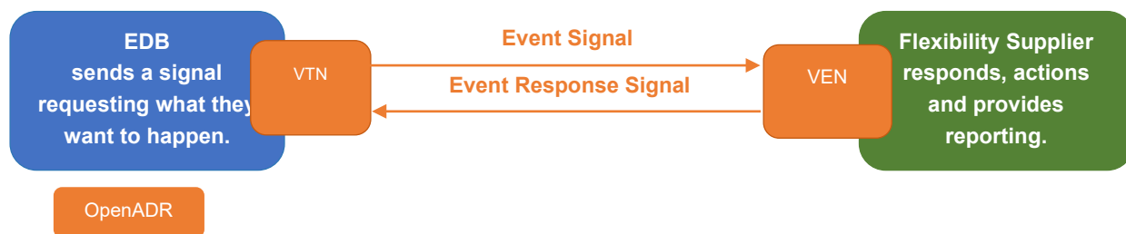
Figure 7: Trial Part B - OpenADR 2.0b communication flow
