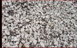
Imported fill GAP40 3% cement
