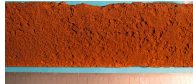
Figure 1 - Bar A metal loss 1.77mm
