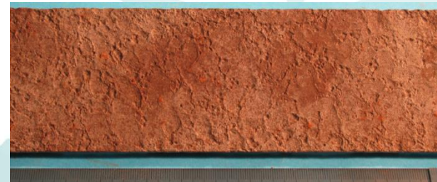
Figure 4 - Bar G Metal loss 0.85mm
