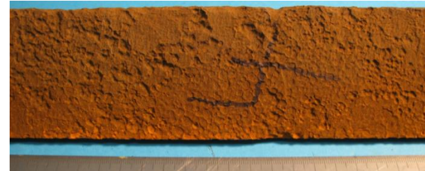
Figure 2 - Bar C Metal loss 1.48mm
